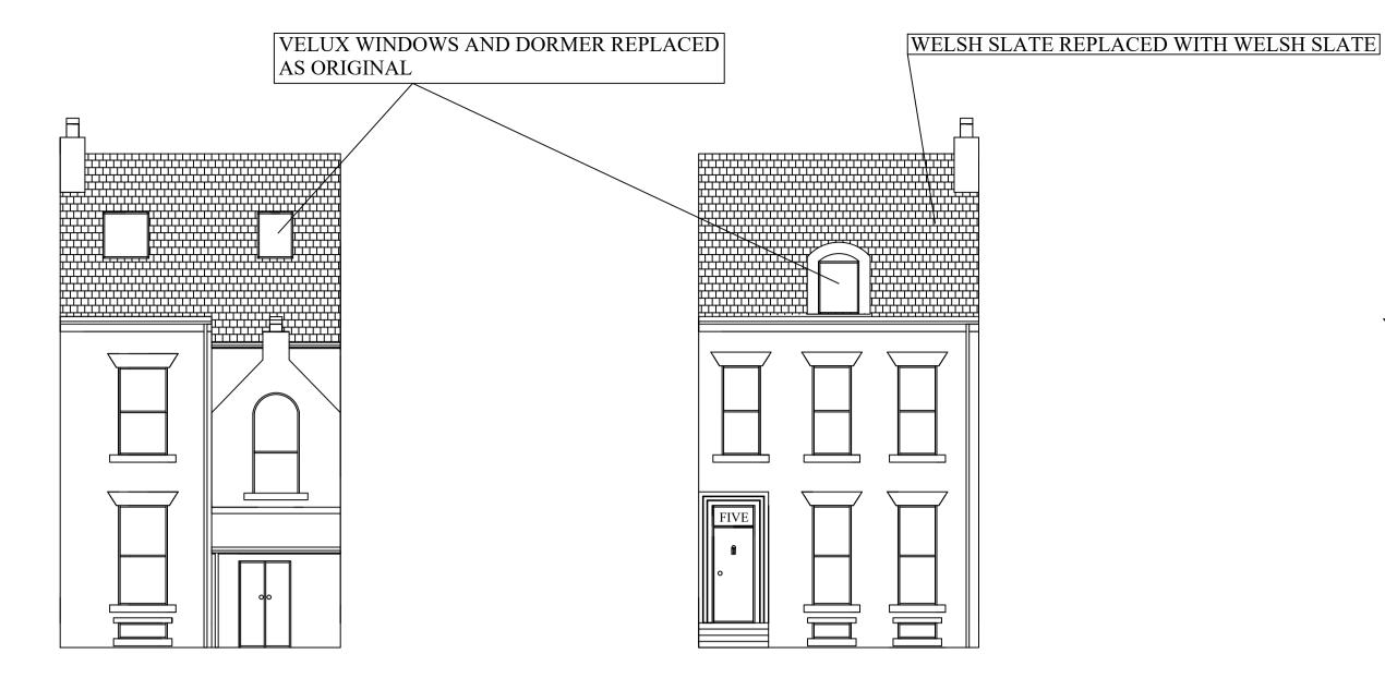
PROPOSED REAR ELEVATION PROPOSED FRONT ELEVATION
